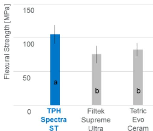
Figure 1 Flexural strength in 4-point bending after 2 weeks of water storage (Belli R and Lohbauer U, 2015)<sup>1</sup>
