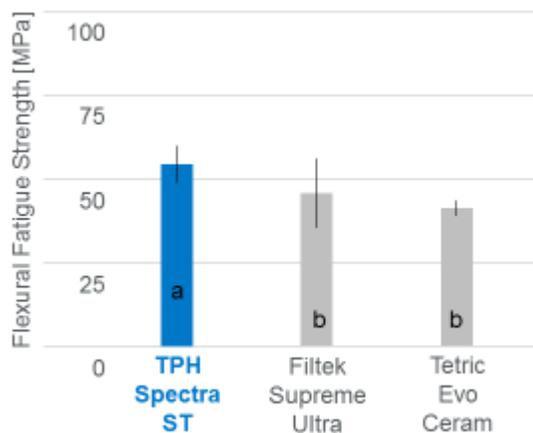
Figure 2 Flexural fatigue strength in 4-point bending (Belli R und Lohbauer U, 2015)<sup>1</sup>
