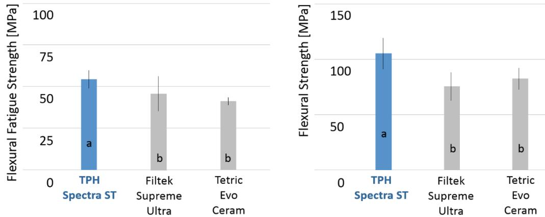
**Fig. 1** Flexural strength in 4-point bending after two weeks of water storage (left) and after fatigue loading (right). Different letters indicate significant differences (Belli R & Lohbauer U, 2015)
