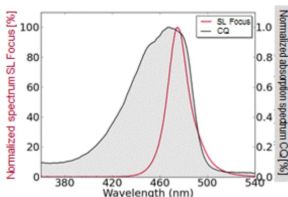
**Figure 2** Normalized absorption spectrum CQ (grey) and emission spectrum SL Focus (red).
