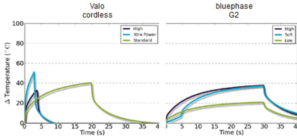
**Figure 16** Surface temperature increase of different curing modes
