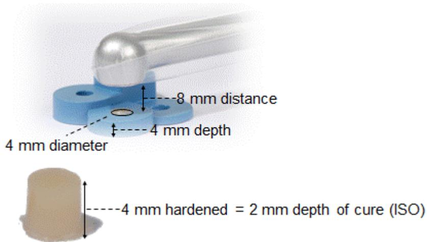
**Figure 5** Depth of cure at 8 mm distance
